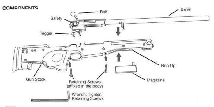
SAFETY SETTING (Always set the safety lever to safe position before firing)
