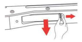
Remove the magazine by pressing the magazine release and pulling the magazine out.
