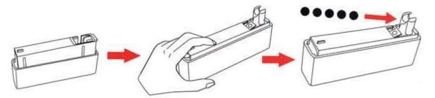
Press the Magazine and load the BB's, maximum of 30 BB's. Do not overload the Magazine. Reinsert the Magazine into the gun, until a "Click" is heard.
