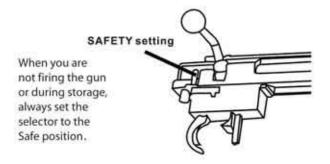
When the safety lever is set to the "On" position, the trigger will not move. Please do not pull the trigger, otherwise you may damage the gun.
